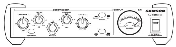
The Samson C com opti optical compressor utilizes a unique photo cell design which produces a classic sound while handling the job of gain management. Here are some of its main features:
