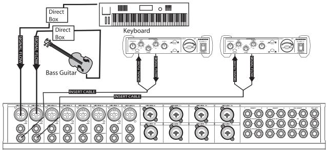
In this example, two C com opti's are used individually to compress the signal of the bass and keyboard tracks. The C comopti's are connected to the mixer's insert points using a standard 1/4-inch insert "Y" cable. See page 13 for a detailed wiring diagram.
