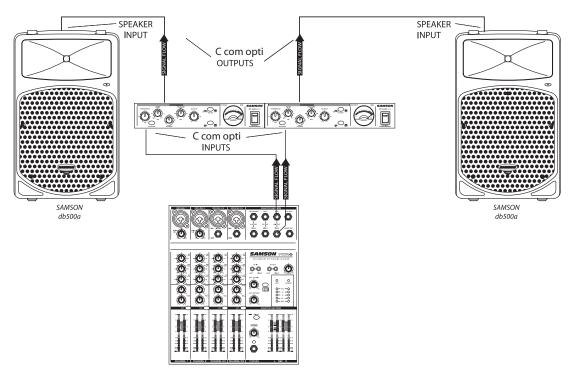
In this example, two C com opti's are connected, "in-line" between the mixer and the powered speakers, thereby compressing the full range signal from the mixer. The STEREO LINK on both units are connected together using a standard 1/4-inch instrument cable.
