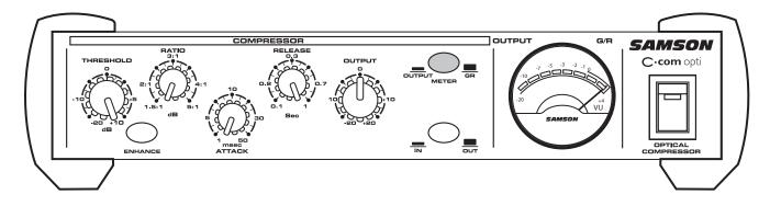
COMPRESSOR THRESHOLD ENHANCER SWITCH RATIO ATTACK RELEASE METER SWITCH OUTPUT LEVEL
